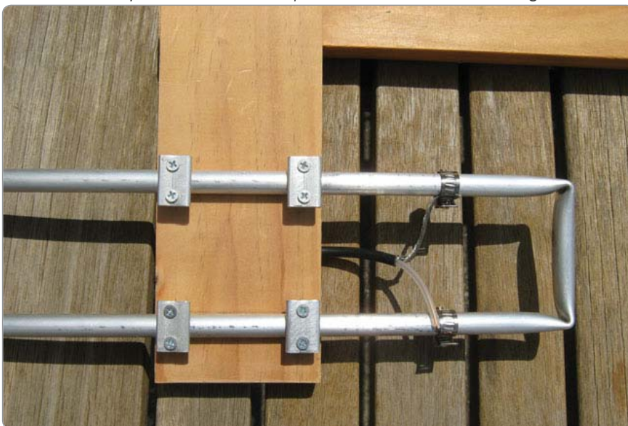
Photo 4: Close up of the antenna feedpoint and an alternate mounting method.
