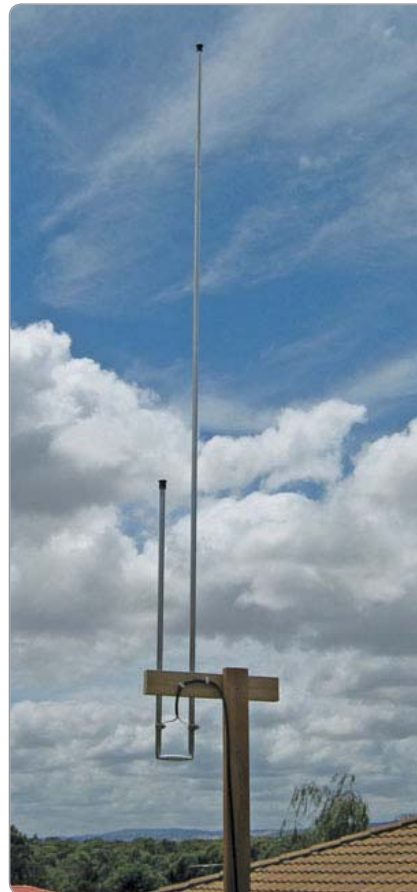
Photo 1: The completed J-pole antenna.
